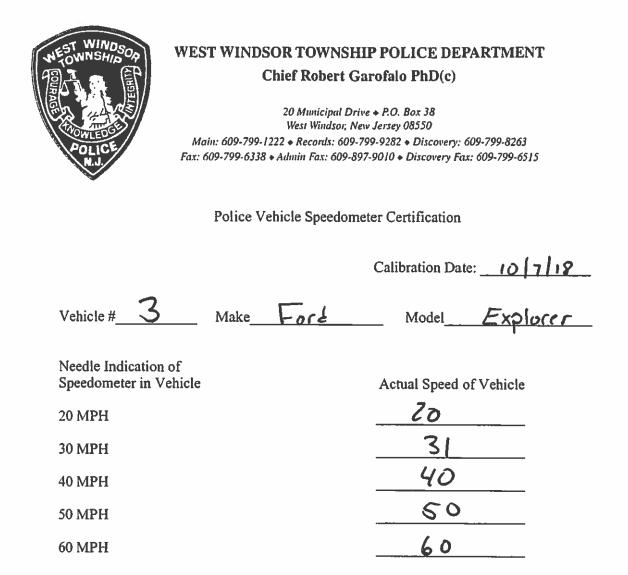
The above listed vehicle's speedometer has been checked for accuracy using a Laser Technology Inc LTI 20/20 TruSpeed S speed detection instrument (serial number TJ001479)
